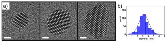
Fig. 2 (a) High-resolution TEM micrographs of Pt nanoparticles, showing crystalline structure and surface faceting (scale bars: 1 nm). (b) Size distribution of Pt nanoparticles (normal distribution) obtained by TEM imaging and automated image analysis, assuming circular nanoparticle diameters.
