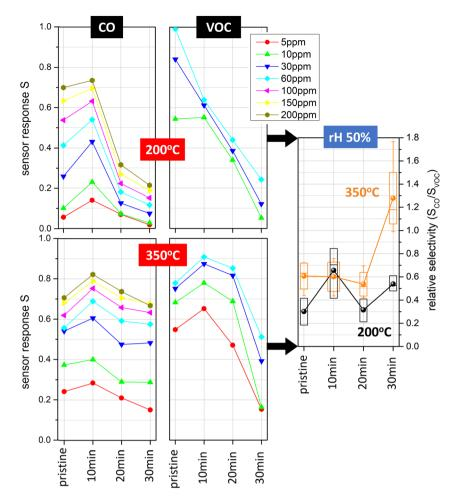
Fig. 4 Sensor response S to CO (left) and VOC (right) of pristine and Pt-decorated SnO<sub>2</sub> sensors (nanoparticle deposition times 10 min, 20 min, 30 min) at 50% relative humidity (rH) and operation temperatures of 200 °C (top row) and 350 °C (bottom row). The relative selectivity (averaged in the concentration range 5-60 ppm) of CO response over VOC response is shown in the right graph.
