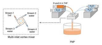
Fig. 11 Schematic representation of the flash nanoprecipitation method utilised by Yu et al. to prepare PNPs and nanofibers. Adapted under CC-BY 4.0 License. 123
