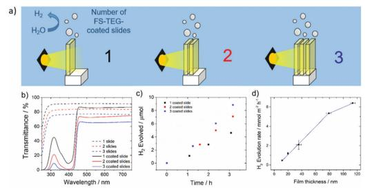
Fig. 22 (a) Schematic diagram of **FS-TEG** coated glass slides stacked in series; (b) UV-vis transmittance spectra of slides stacked in series; (c) hydrogen evolved of stacked slides under visible light; (d) hydrogen evolution rates of **FS-TEG** films at varying thicknesses. Reprinted under CC-BY 3.0 License.<sup>43</sup>
