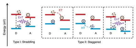
Fig. 5 Schematic representations of energy level alignment of type-I and type-II semiconductor heterojunctions and energy transfer (EnT), electron transfer (ET), and hole transfer (HT) between donor (D) and acceptor (A) semiconductors. N.B. the arrow representing energy transfer does not represent a radiative process.<sup>11</sup>
