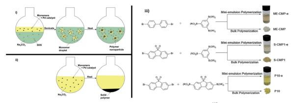
Fig. 13 Mini-emulsion polymerisation utilised by Aitchison et al. Reproduced under CC-BY 3.0 License. 113
