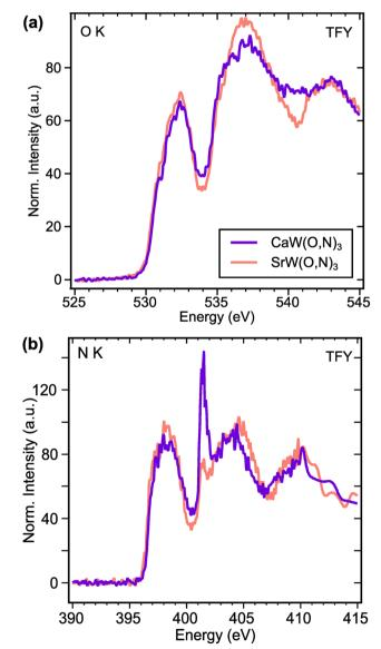
Fig. 5 (a) Oxygen and (b) nitrogen K-edge XAS spectra of  $CaWO_2N$  and  $SrWO_2N$  perovskite powder samples measured in total fluorescence yield. Intensities are area-normalized between 528–545 eV for O K-edge and 394–410 eV for N K-edge.
