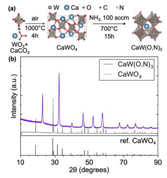
Fig. 1 (a) Synthesis route for CaW(O,N)<sub>3</sub> consisting of calcination of WO<sub>3</sub> and CaCO<sub>3</sub> precursors followed by ammonolysis of the scheelite CaWO<sub>4</sub> intermediate. (b) XRD patterns of intermediate scheelite phases, CaWO<sub>4</sub> and CaW(O,N)3, demonstrating their differing crystal structures. CaWO4 reference is provided.<sup>29</sup> Crystal structure images generated using VESTA.<sup>30</sup>
