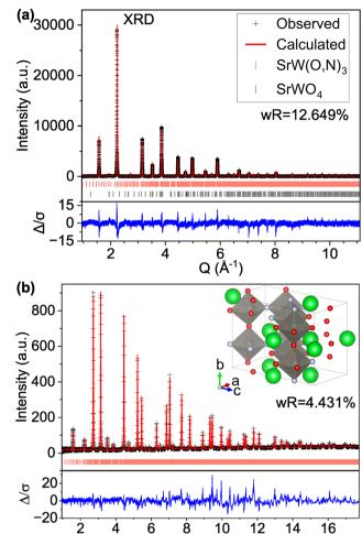
Fig. 4 Rietveld refinement of SrW(O,N)<sub>3</sub> (a) synchrotron XRD and (b) ND patterns using a 40-atom P1 structure suggested by our theory-based approaches (model S-II)
