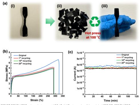
Fig. 5 Recycling of PEDOT: PSS/PU/PEG using a hot press at 100 °C. (a) Photographs of the original PEDOT: PSS/PU/PEG sample (i) after being cut into small pieces (ii) and after remolding by hot-pressing (iii). (b) Comparison of tensile stress–strain curves for the PEDOT: PSS/PU/PEG sample before and after recycling (1, 10 and 20 times). (c) Current vs. time plot before and after recycling (1, 10 and 20 times) (applied voltage of 0.2 V).
