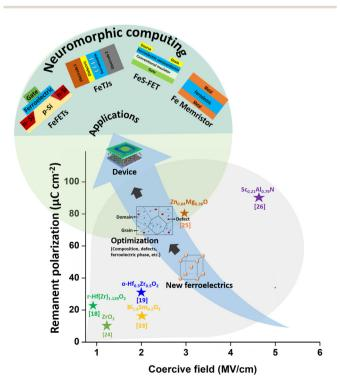
Fig. 3 New ferroelectric materials and their possible applications. o- and r- indicate orthorhombic and rhombohedral phases, respectively.
