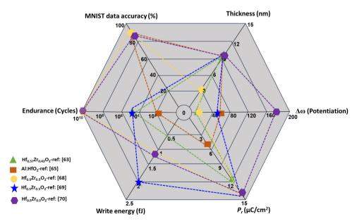
Fig. 5 Performance of HfO<sub>2</sub>- and ZrO<sub>2</sub>-based FeFETs for different key parameters that are required for neuromorphic computing devices.
