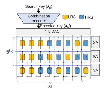
Fig. 2 Schematic of N-CECAM (N = 4). The search key  $\mathbf{k}_b$  is encoded into a 2N-long binary array  $\emph{\textbf{k}'}_{b}$  by the combination encoder. Each bit of the encoded key represents the corresponding voltage at search lines (low voltage for 0s and high voltage for 1s). Matching search is obtained at the lowest matching current.
