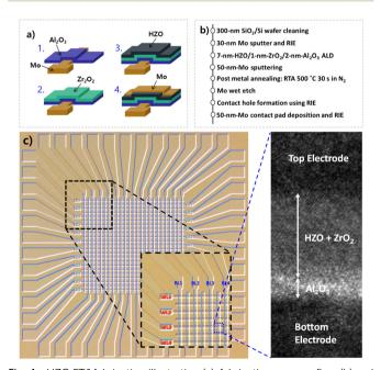
Fig. 4 HZO FTJ fabrication illustration (a), fabrication process flow (b) and top view image and cross-sectional transmission electron microscopy (TEM) image of the HZO FTJ crossbar array (c).
