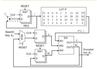
Fig. 3 Block diagram of the combination encoder to convert a search key  $\mathbf{k}_{b}$  to a 2N-long key  $\mathbf{k}_{b}'$  with N 0s and N 1s.
