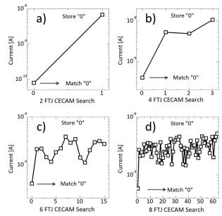
Fig. 10 Searching results of N-CECAM based on HZO FTJ ( $100 \times 100 \ \mu m^2$ ) crossbar arrays with same stored information of "0" with different N values: N=1 (a), N=2 (b), N=3 (c), and N=4 (d).
