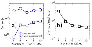
Fig. 11 Match current and mean unmatch current at different CECAM sizes (a) and unmatch/match current ratio with the scaling CECAM size (b).
