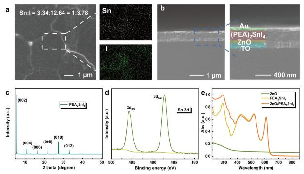
Fig. 2 (a) Top-view SEM image of PEA<sub>2</sub>SnI<sub>4</sub> and mapping images for the corresponding elements (Sn and I). (b) Cross-sectional image of the PEA<sub>2</sub>SnI<sub>4</sub>/ ZnO device. (c) XRD pattern of PEA<sub>2</sub>SnI<sub>4</sub> film. (d) XPS spectra of PEA<sub>2</sub>SnI<sub>4</sub>: Sn 3d. (e) Absorption spectrum of ZnO, PEA<sub>2</sub>SnI<sub>4</sub>, and the PEA<sub>2</sub>SnI<sub>4</sub>/ZnO films.
