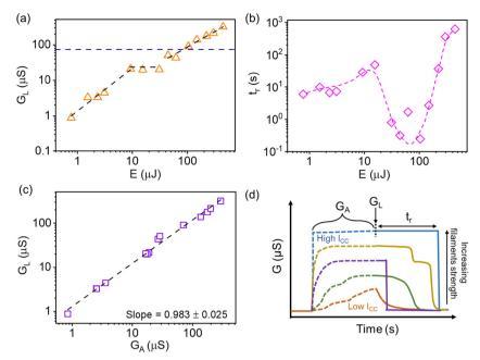
Fig. 4 Analysis of the G profile. (a) Variation of  $G_1$ , and (b)  $t_r$  as a function of the electrical energy stress (E) on the device. (c) Variation of  $G_1$  with  $G_2$ . (d) Schematic of a typical G profile (G evolution during pulsing and retention after pulsing) visualised at different ranges of ICC under similar pulsing conditions ( $V_P \sim 1 \text{ V}, V_R \sim 10 \text{ mV}, t_i \text{ and } t_w \sim 50 \text{ ms}$ ).
