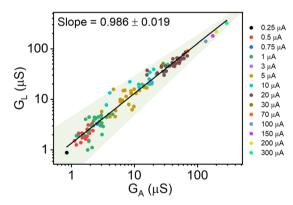
Fig. 6 Correlation of  $G_L$  with  $G_A$  of the G profile with varied  $N_p$  in the  $I_{CC}$ range of 0.25 to 300  $\mu$ A. Data are sourced from Fig. 4 and 5.
