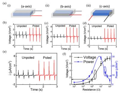
Fig. 3 (a) Schematic of electrode connection in (i) a-, (ii) b- and (iii) c-axis on a single crystal of 1 with corresponding voltage vs. time response in poled and unpoled device along (b) a-, (c) b- and (d) c-axis under cyclic load of 6 N. (e) Current vs. time response of poled and unpoled device along b-axis. (f) Normalized voltage vs. resistance and power density curve along the b-axis.
