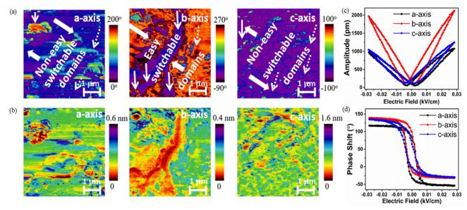
Fig. 2 (a) Vertical PFM phase images recorded on a single crystal of  $\bf 1$  oriented along a-, b- and c-axis and (b) corresponding amplitude images showing the different domains, (c) amplitude vs. electric field butterfly loop, (d) phase shift vs. electric field hysteresis loop along the three directions (applied voltage is normalized with respect to electric field).
