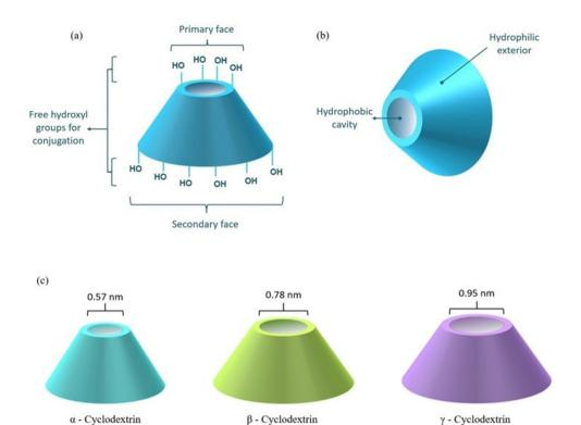
Fig. 1 Toroidal architectures of cyclodextrins: (a) primary and secondary faces of cyclodextrin with free hydroxyl groups for potential structural modification with different groups, (b) the less hydrophilic cavity and hydrophilic exterior of cyclodextrin and (c) the cavity size of different cyclodextrins.
