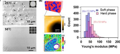
Fig. 4 (a) SEM images of PIBXA-TEP (20 wt%) at 25 and 50 °C. (b) Height and Young's modulus mapping of PIBXA-TEP (20 wt%) measured by AFM. The dashed line in modulus mapping is a boundary between the inner soft and outer hard phases to calculate each average modulus. The average modulus is calculated by Gaussian fitting of the histogram.
