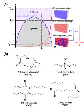
Fig. 1 (a) Thermodynamic phase diagram with a demixing curve and a  $T_{\alpha}$ curve for a two-component system showing phase separation-induced glass transition. If a polymeric material does not show any phase separation, it will show the glass transition at  $T_{{
