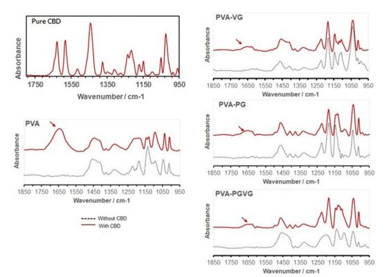
Fig. 4 FTIR spectra confirming the presence of CBD in the hydrogels (arrows). Adding PG and VG attenuated the absorption of CBD on the hydrogel surface.
