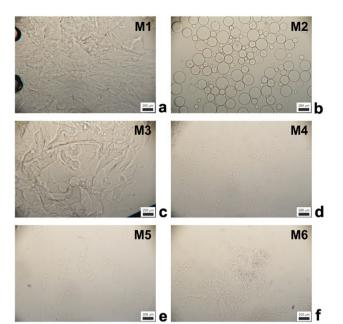
Fig. 1 Light microscopy images of P2HPG-Tyr microgels swollen in H<sub>2</sub>O prepared by HRP/H<sub>2</sub>O<sub>2</sub>-mediated microgelation in inverse suspension and stabilized with SPAN 80 without (a) and with pre-emulsification (b), TWEEN 85 without (c) and with pre-emulsification (d), and AOT without (e) and with pre-emulsification (f).
