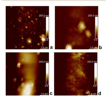
Fig. 3 PF-QNM topography height images of P2HPG-Tyr microgels on mica substrate (a), (b) and glass substrate (c), (d), swollen in Q-H $_2$ O (a), (c), and PBS buffer (b), (d).
