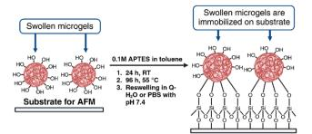
Scheme 2 Immobilization of swollen P2HPG-Tyr microgels on APTES-modified mica and glass substrates (created with BioRender.com).
