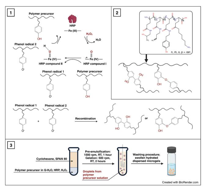
Scheme 1 Microgelation of P2HPG-Tyr polymer precursor in inverse suspension by HRP/H2O2-mediated crosslinking. (1) Mechanism of the HRP/ H<sub>2</sub>O<sub>2</sub>-mediated crosslinking, (2) structures of P2HPG-Tyr polymer precursor and P2HPG-Tyr crosslinked microgel, and (3) a schematic illustration of the microgelation process.
