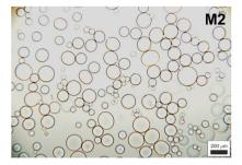
Fig. 2 Light microscopy image of M2 microgels swollen in PBS buffer (pH 7.4, room temperature) prepared by HRP/H<sub>2</sub>O<sub>2</sub>-mediated microgelation in inverse suspension including pre-emulsification and stabilized with SPAN 80
