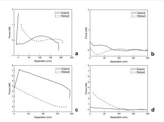
Fig. 5 Force-separation curves of swollen M4 on mica (a), (b) and glass (c), (d) substrates in Q-H<sub>2</sub>O (a), (c) and PBS buffer with pH 7.4 (b), (d).
