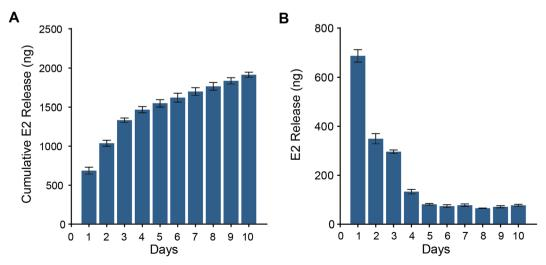
Fig. 3 PHS hydrogel sustained release of E2 over ten days. (A) Cumulative release of E2 over ten days. (B) Daily release of E2 over the ten-day period.
