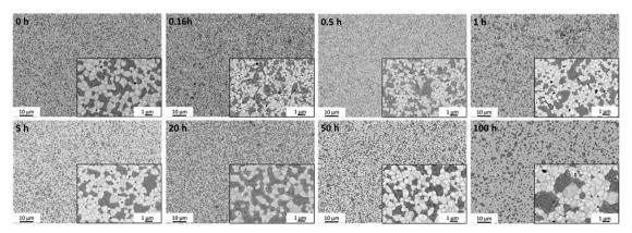
Fig. 3 BSE-images of 60CGO20-FCO surface morphology of the samples sintered at 1200 °C with two magnifications.
