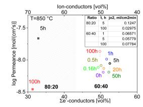
Fig. 15 Comparison of the final permeation performance permeance of CGO20-FCO composite with ratio 60:40 and 80:20 sintered with various dwell times depending on the volume fraction of e--conducting phases
