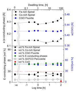
Fig. 2 Lattice parameter and volume fraction of observed phases in 60CGO20-FCO composites sintered at  $1200\,^{\circ}\text{C}$  (solid lines are a guide to the eve).
