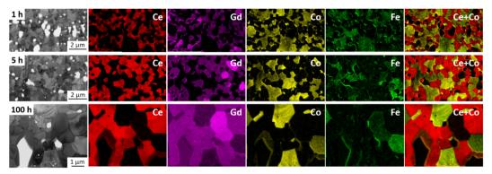
Fig. 6 Energy-filtered TEM (EFTEM) analysis of 60CGO20-FCO composite sintered at 1200 °C for 1 h, 5 h and 100 h, identifying three main phases: Gd-doped ceria (red), Fe/Co-oxide (green) and the GdFeO<sub>3</sub>-based perovskite (bright magenta).
