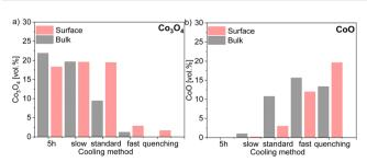
Fig. 11 Volume fraction of 60CGO20-FCO composite subjected different heat treatment and cooling methods in (a) Co<sub>3</sub>O<sub>4</sub> and (b) CoO amount comparison in the bulk and surface.
