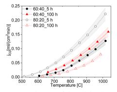
Fig. 16 Oxygen permeation rates of the ceria-based materials with 60:40 and 80:20 ratios sintered at 5 and 100 h (solid lines are a guide
