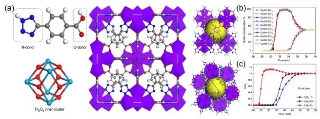
Fig. 5 (a) A Th-MOF (Azole-Th-1) based on Th<sub>6</sub> secondary building unites and tetrazolyl groups. (b) C<sub>2</sub>H<sub>6</sub>/C<sub>2</sub>H<sub>4</sub> (50/50, v/v) binary mixture separation for five cycles. (c) C<sub>2</sub>H<sub>6</sub>/C<sub>2</sub>H<sub>4</sub>/C<sub>2</sub>H<sub>2</sub> (90/9/1, v/v/v) ternary mixture separation. Reproduced with permission from ref. 54. Copyright © 2020, Springer Nature Publishing AG.
