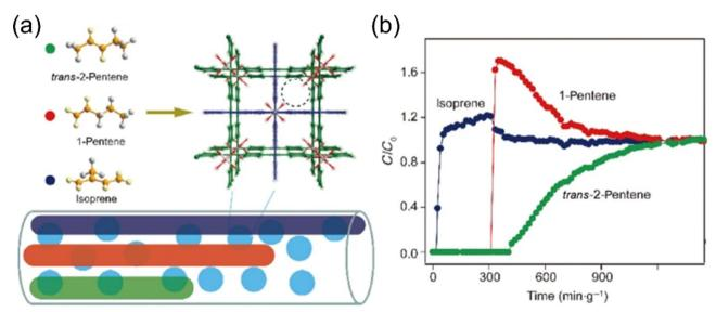
Fig. 12 (a) Schematic diagram of TIFSIX-2-Cu-i and ZU-62 for the separation of trans-2-pentene/1-pentene/isoprene. (b) The breakthrough performance of TIFSIX-2-Cu-i for trans-2-pentene/1-pentene/isoprene/N2 (9%/9%/9%/73%, v/v/v/v) ternary mixtures. Reproduced with permission from ref. 94. Copyright © 2021, Springer Nature Publishing AG
