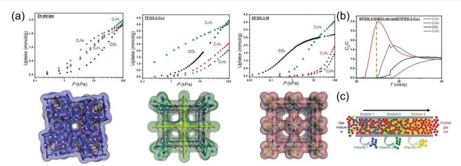
Fig. 9 (a) Structure and adsorption isotherms of three high-performance ultra-porous MOFs. (b) One step separation of high purity  $C_2H_4$  in a four-component hybrid system. (c) Diagram of the synergy of the three MOFs. Reproduced with permission from ref. 4. Copyright © 2019, The American Association for the Advancement of Science.
