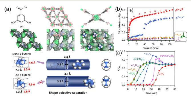
Fig. 11 (a) Structure, channel, and separation of trans-and cis-2-butene of M-gallate. (b) Adsorption isotherms of trans-2-butene, cis-2-butene, 1,3butadiene, 1-butene, iso-butene, n-butane, and iso-butane on Co-gallate at 298 K. (c) Mixture breakthrough curves on Mg-gallate for 1,3-butadiene/1butene/iso-butene/n-butane/iso-butane/trans/cis-2-butene/He (20/10/10/5/1/2/50) at 298 K. Reproduced with permission from ref. 91. Copyright (i) 2020, American Chemical Society
