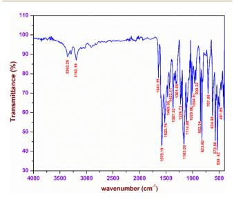
Fig. 3 FTIR spectrum of DMMA.
