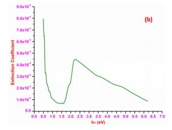
(a) Bandgap and (b) extinction coefficient vs. photon energy
