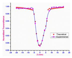
Fig. 15 Open aperture plot of the DMMA crystal
