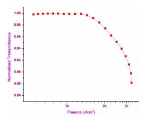
Fig. 16 Optical limiting behaviour of DMMA crystal
