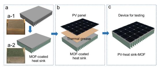
Fig. 2 Schematic of device assembly processes. (a) the MOF coating process; (a-1) photo of the heat fins before spray coating; (a-2) photo of the heat fins after spray coating with Cr-soc-MOF-1. (b) The device assembling process. (c) The as-assembled devices for testing
