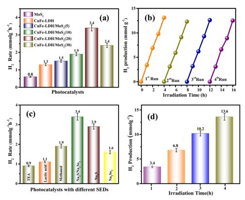
Fig. 5 (a) Histogram showing various photocatalysts' varying rates of  $H_2$  creation, (b) reclaimable nature of CuFe-LDH/MoS<sub>2</sub>(20), (c) various sacrificial agents employed to measure the  $H_2$  creation rate for the CuFe-LDH/MoS<sub>2</sub>(20) semiconductor and (d) time on stream of hydrogen yield up to 4 hours of CuFe-LDH/MoS<sub>2</sub>(20).
