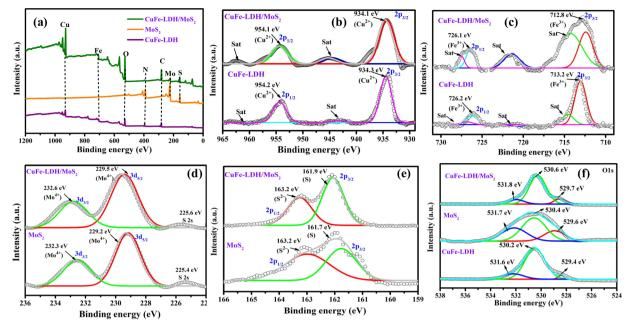
Fig. 4 The XPS spectra of CuFe-LDH, MoS<sub>2</sub>, and CuFe-LDH/MoS<sub>2</sub>: (a) survey spectra, (b) Cu 2p, (c) Fe 2p, (d) Mo 3d, (e) S 2p and (f) O 1s.
