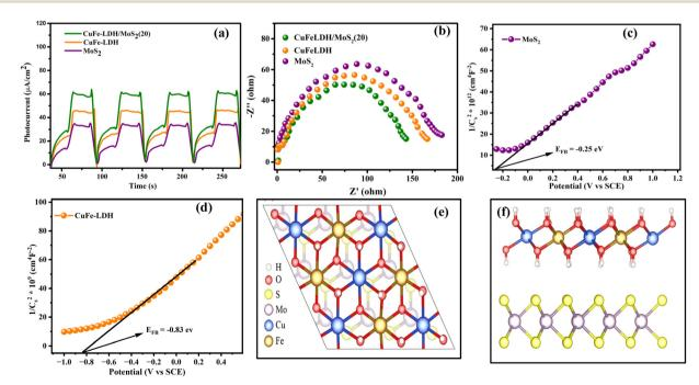
Fig. 6 (a) Response of transient photocurrent, (b) electrochemical impedance spectra of  $MoS_2$ , CuFe-LDH, and  $CuFe-LDH/MoS_2(20)$ , (c), (d) Mott-Schottky plots of  $MoS_2$  and CuFe-LDH, (e) top view and (f) side view of the  $CuFe-LDH/MoS_2$  heterostructure.
