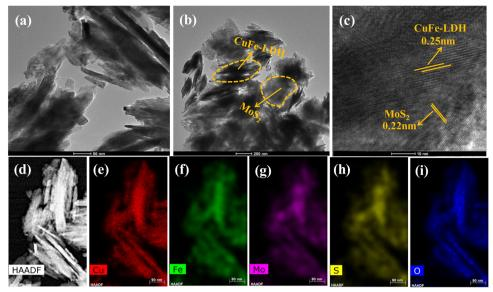
Fig. 2 TEM images of (a) CuFe-LDH, (b) CuFe-LDH/MoS<sub>2</sub>(20), (c) HR-TEM image of CuFe-LDH/MoS<sub>2</sub>(20) and (d)-(i) HAADF-STEM and elemental analysis of CuFe-LDH/MoS<sub>2</sub>(20).
