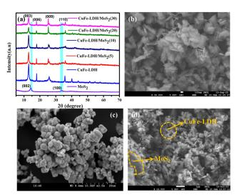
Fig. 1 (a) PXRD spectra, and FESEM images of (b) CuFe-LDH, (c) MoS<sub>2</sub>, and (d) CuFe-LDH/MoS<sub>2</sub>.
