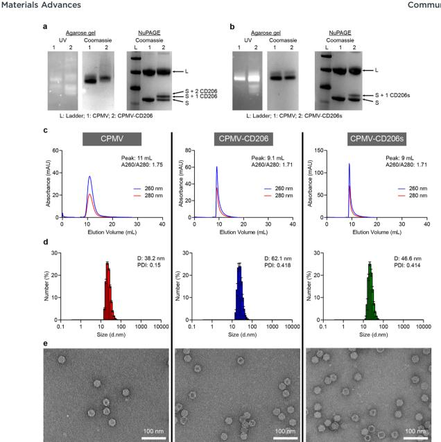
Fig. 1 Characterization of modified CPMV particles. (a) and (b) Comparison of CPMV to (a) CPMV-CD206 and (b) CPMV-CD206s by agarose gel electrophoresis and NuPAGE. (c) Analysis of CPMV, CPMV-CD206, and CPMV-CD206s by size exclusion chromatography. (d) Analysis of CPMV, CPMV-CD206. CD206, and CPMV-CD206s by dynamic light scattering. (e) Transmission electron microscopy images of CPMV, CPMV-CD206, and CPMV-CD206s.
