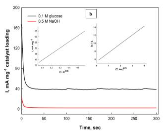
Fig. 12 (a) Repeated cyclization of the Ni(II)–SB/C electrode in 0.5 M NaOH +0.1 M glucose, and (b) chronoamperometry of the same electrode at 0.72 V and the inset plots represent I and 1/square root of time (left) and the relationship of  $I_{\rm C}/I_{\rm L}$  and square root of time (right).
