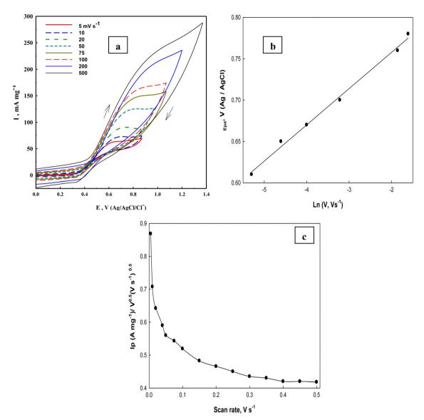
Fig. 11 (a) Cyclic voltammograms of Ni(II) – SB/C electrode in 0.5 M NaOH + 0.1 M glucose at different scan rates, (b) the relationship between the natural logarithms of scan rates and the peak potentials, and (c) the  $I_p/v^{0.5}$  vs. scan rates relationship for glucose electrooxidations obtained at the Ni(II) – SB/C electrode.
