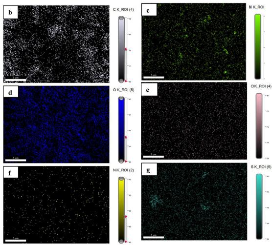
(a) EDX analysis with the inset data of wt% and at% of each element, and (b)-(g) elemental mapping of each element of the prepared Ni(II)-SB complex.
