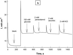
Fig. 14 Chronoamperometry of electroxidation of glucose at 0.72 V in 0.5 M NaOH in the presence of (a) different concentrations of glucose from 1 mM to 100 mM, with the inset calibration plot and (b) different interfering species.
