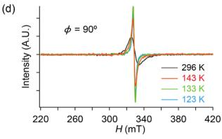
Fig. 5 Comparison of the T-dependent ESR spectra between different orientations ( $\theta$ ,  $\phi$  = 0 and 90°) and between different rotation axes (b- and c-axes) of  $\alpha\text{-ET}_2I_3.$  The sample (single crystal) was rotated around the baxis (a), (b) and the c-axis (c), (d) with the indicated magnetic-field-angle  $\theta$ and  $\phi$ , respectively.  $\boldsymbol{H} \| \boldsymbol{a}$ -axis when  $\theta = 0^{\circ}$  and  $\phi = 0^{\circ}$ .
