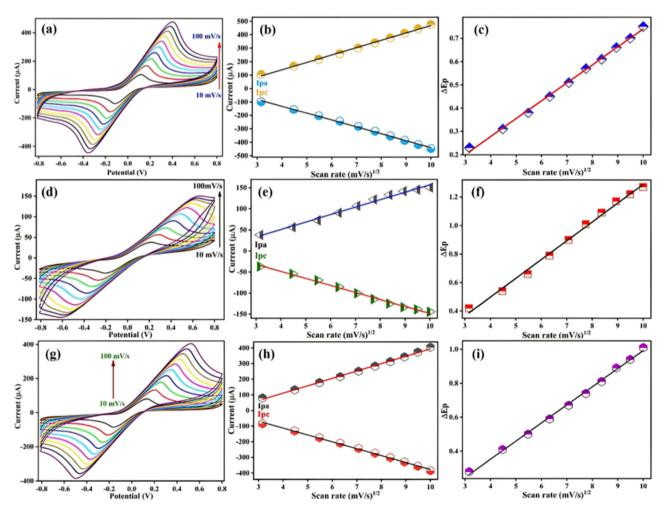
Fig. 5 Scan rate analysis of different electrodes: (a) SPE, (d) BSA/anti-CYFRA21-1/SPE, and (g) BSA/anti-TP53/SPE in PBS.  $I_{\rm pa}$  and  $I_{\rm pc}$  peak current curves of (b) SPE, (e) BSA CYFRA21-1/SPE and (h) BSA/anti-TP53/SPE electrodes, respectively, with the square root of scan rates. Changes in peak potential ( $\Delta E_{\rm p}$ ) versus the square root of scan rates for (c) SPE, (f) BSA/CYFRA21-1/SPE and (i) BSA/anti-TP53/SPE bioelectrodes, respectively.
