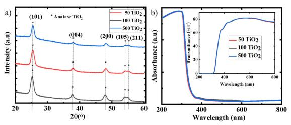
Fig. 2 (a) XRD spectra and (b) absorption spectra with transmission spectra of 50 TiO2, 100 TiO2 and 500 TiO2 as the inset image.
