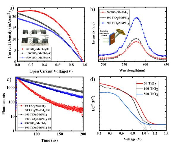
Fig. 7 (a) IV characteristics of CPSCs with 50 TiO2, 100 TiO2 and 500 sintered TiO2 as the ETL; (b) PL spectra and (c) TRPL spectra of MaPbI3 films deposited on 50 TiO2, 100 TiO2 and 500 sintered TiO2. (d) Mott-Schottky analysis at 1 kHz for the TiO2/MaPbI3 carbon heterojunction solar cell.
