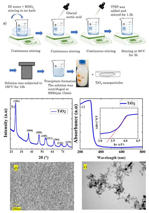
Fig. 1 (a) Schematic representation of uniformly dispersed anatase TiO<sub>2</sub> sol and nanoparticle synthesis, (b) XRD spectra, (c) absorbance spectra (d) FE-SEM images and (e) TEM of TiO<sub>2</sub> films fabricated from TiO<sub>2</sub> sol.
