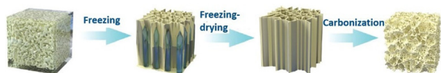
Fig. 12 Schematic illustration of the fabrication of N-MPC. Reproduced from ref. 88 with permission from Wiley-VCH, Copyright [2021].
