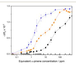
Fig. 4 Relative frequency shift for DUT-4(Al)/MIL-100(Fe)@QCM (orange circles), DUT-4(Al)@QCM (blue stars), MIL-100(Fe)@QCM (black squares), and uncoated QCM (grey triangles) *versus* increasing  $\alpha$ -pinene concentration. Error bars represent the standard deviations over cycling experiments. Lines are guides for the eyes.
