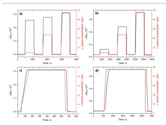
Fig. 3 Real-time sensor response of a) DUT-4(Al)@QCM and b) MIL-100(Fe)@QCM to multiple changes of  $\alpha$ -pinene concentration from 2 ppm to 5 ppm, 24 ppm, and 47 ppm and vice versa, with a highlight of the kinetics of the last cycle (2 ppm-47 ppm-2 ppm) for c) DUT-4(Al) @QCM and d) MIL-100(Fe)@QCM.
