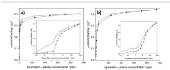
Fig. 1 Gravimetric sorption isotherms of  $\alpha$ -pinene recorded at 303 K on a) DUT-4(Al) and b) MIL-100(Fe) powder, increasing (filled black and decreasing (empty black squares)  $\alpha$ -pinene concentration. Insets show the isotherms on a semi-logarithmic basis. Lines are guides for the eyes.
