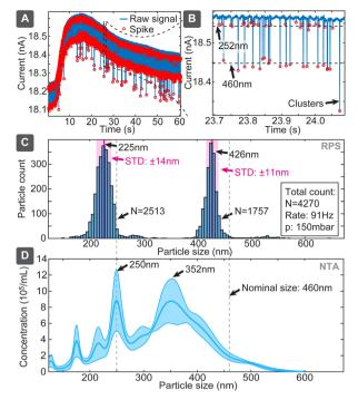
distribution and concentration measurement polydisperse samples represented by mixture of 252 nm and 460 nm particles in respective concentrations of  $5.7 \times 10^9$  and  $2.9 \times 10^9$ particles per mL. (A) Raw measured signal (blue) with detected particles indicated with red. (B) Same in enlarged scale. (C) Histograms of populations of spikes corresponding to both sizes of particles, while (D) shows NTA measurement of mixture of same particles (108 particles per mL each).
