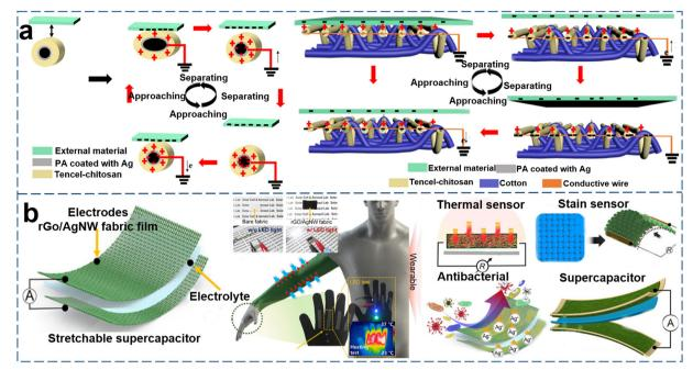
Fig. 11 (a) Structure and working principle of friction nanogenerator, <sup>187</sup> Copyright 2021 American Chemical Society; (b) wearable supercapacitors and human motion sensors, 191 Copyright 2021 American Chemical Society.
