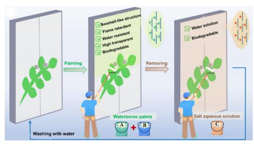
Fig. 6 Switchable waterborne coatings, <sup>129</sup> Copyright 2023 American Chemical Society.
