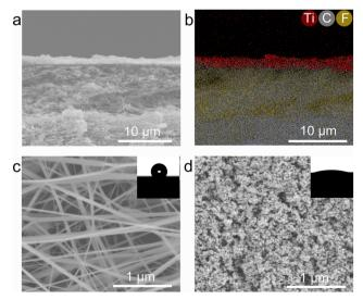
Fig. 2 Structural characterization of the Rh/TiO2-GDL. (a) Crosssectional SEM image and (b) corresponding EDS mapping of Rh/TiO<sub>2</sub>-GDL; top-view SEM images of (c) pristine GDL porous substrate and (d) immobilized Rh/TiO2 photocatalyst layer. Inserts in (c) and (d) show photographs of water droplets on each sample.
