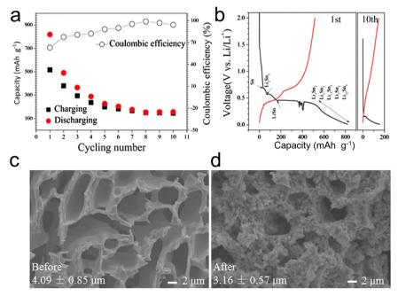
Fig. 14 (a) Cycling performance and (b) charge/discharge curve of the porous Sn dealloyed from Al<sub>80</sub>Sn<sub>20</sub>; SEM images of the porous Sn structure before (c) and after (d) the lithiation/delithiation process. Reprinted with permission from ref. 127. Copyright 2015, Springer.
