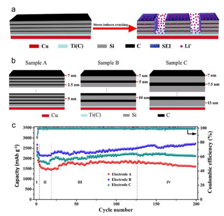
Fig. 12 (a) Schematic illustration of Si/C multilayer blocks formed by stress; (b) schematic illustration of Si/C multilayer films structure; (c) cycling performance of electrodes A–C at a current density of 300 mA  $g^{-1}$ . Reprinted with permission from ref. 123. Copyright 2019, American Chemical Society.
