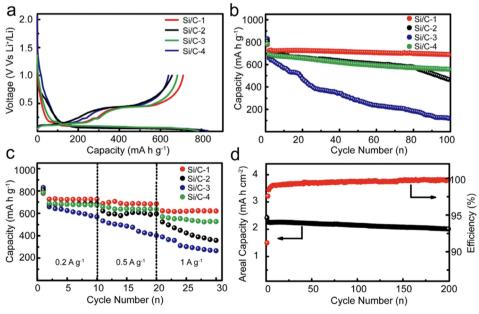
Fig. 10 (a) The first charge and discharge profiles; (b) the cycling stability; (c) rate capability of different Si/C anodes; (d) high areal mass loading test and coulombic efficiency of the Si/C-1 anode. Reprinted with permission from ref. 117. Copyright 2016, WILEY-VCH Verlag GmbH & Co. KGaA, Weinheim.
