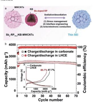
Fig. 13 (a) Schematic illustration and (b) cycling performance in carbonate electrolyte and localized highly concentrated ether electrolyte (LHCE) of hierarchical micro/nanostructured Sb<sub>x</sub>-RP<sub>70-x</sub>/KB-MWCNTs. Inset: first charge/discharge curve in two electrolytes. Reprinted with permission from ref. 125. Copyright 2021, American Chemical Society.
