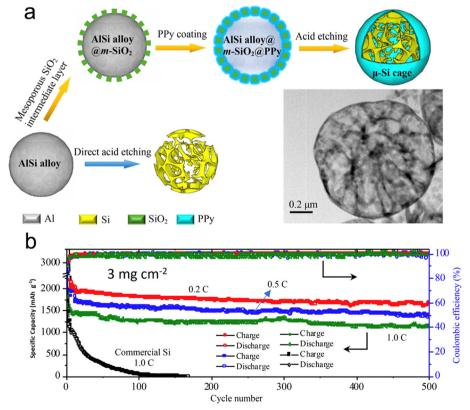
Fig. 11 (a) Scalable synthesis of the  $\mu$ -Si cage using AlSi microspheres as precursor by a chemical method (inset shows the TEM image of the  $\mu$ -Si cage); (b) cycling performance of the battery with a μ-Si cage as anode with loadings of 3 mg cm<sup>-2</sup>. Reprinted with permission from ref. 122. Copyright 2019, American Chemical Society.
