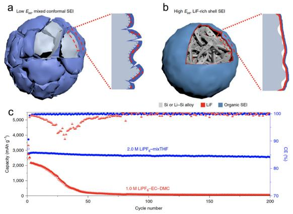
Fig. 3 Schematic of the cycled alloy anode with an organic, low  $E_{int}$  and non-uniform (a) and an inorganic, high  $E_{int}$  and uniform (b) Li alloy-SEI interface; (c) cycling stability and CEs of SiMPs cycled in 2.0 M LiPF<sub>6</sub>-mixTHF and 1.0 M LiPF<sub>6</sub>-EC-DMC electrolytes at C/5. Reprinted with permission from ref. 66. Copyright 2020, Springer Nature.
