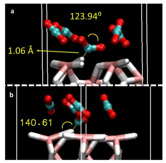
Fig. 3 Details of the geometric parameters of (a) adsorbed CO<sub>2</sub> bending angle and C-H4 distance and (b) Mg2-H4-C contact angle related to the  $CO_2$  (n = 1) molecule behaviour in the structure of 5 adsorbed CO2 molecules.
