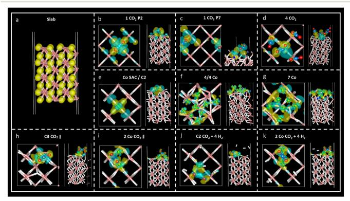
Fig. 5 Charge density difference maps ( $\rho_{\text{system}}$  –  $\rho_{\text{Slab}}$  –  $\rho_{\text{Co}}$  –  $\rho_{\text{gas}}$ ) for the most stable structures (a–k) with the isosurface value of 0.005e. The yellow region represents charge density accumulation, while the blue region represents charge depletion.
