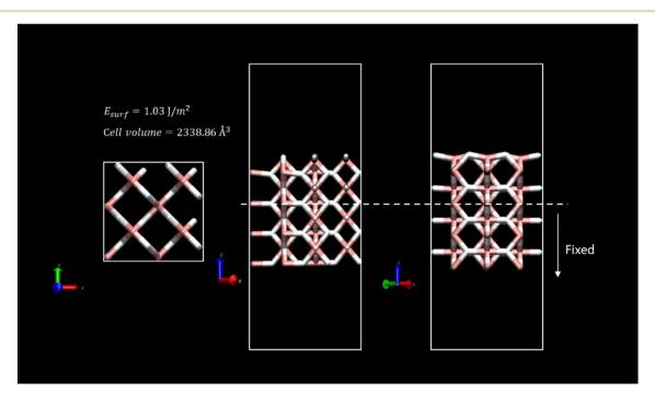
Fig. 1 Top- and two-side-view representations of the system used in the simulations. The (0 0 1) surface energy and total volume of the optimized slab after calculation are depicted. Atom colour code: (white) hydrogen, (pink) magnesium.
