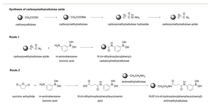
Fig. 13 Two different routes for the grafting of boronic acid onto cellulose proposed by Weith et al. This figure has been reproduced from ref. 55 with permission from the American Chemical Society, copyright 1970.
