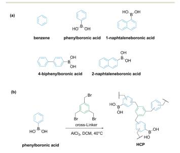
Fig. 11 (a) Functional monomers for the manufacture of the polymers; (b) Friedel–Crafts method to synthesize boronate containing microporous resins. <sup>61</sup>
