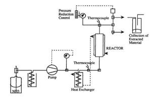
Fig. 12 Schematic of the ammonolysis apparatus working with supercritical ammonia. Reprinted with permission from ref. 69. Copyright 1992 Wilev.
