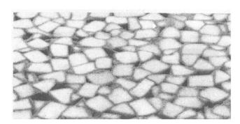
Rebonded foam: homogeneous distribution of the flake-binder mixture. Reproduced with permission from ref. 27. Copyright 2007 Elsevier.
