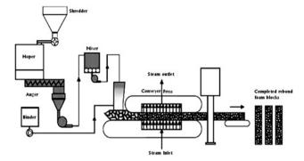
Fig. 8 Schematic of flexible foam re-bonding. Reproduced with permission from ref. 27. Copyright 2007 Elsevier.
