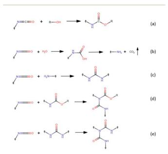
Fig. 1 Reaction between isocyanates and hydroxyl-containing compounds (a), water (b), amine (c), urethane (d), and urea (e).
