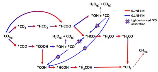
Proposed reaction mechanism over 0.7Ni-TiN and 0.1Ni-TiN
