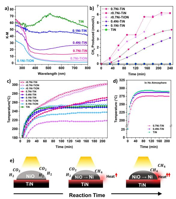
Fig. 2 (a) UV-vis absorption spectra for neat TiN, 0.1Ni-TiN, 0.4Ni-TiN, 0.7Ni-TiN and oxidised controls (0.1Ni-TiON, 0.7Ni-TiON); (b) photothermal CH<sub>4</sub> production by the various samples; (c) corresponding temperature profiles under photothermal conditions (Xe lamp at 20A setting); (d) xNi-TiN temperature profiles under inert He atmosphere ( $\sim$ 80 kPa); (e) proposed photothermally-driven *in situ* Ni reduction mechanism.
