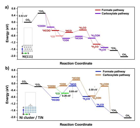
Fig. 5 Calculated free energy profile for methanation under the formate and carboxylate-assisted routes over (a) Ni(111) (0.7Ni-TiN model); and (b) Ni cluster/TiN (0.1Ni-TiN model); modelled cell shown as inset.
