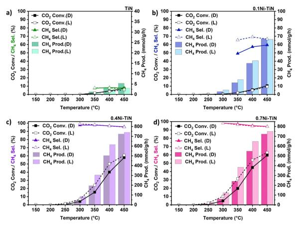
Fig. 3 CO<sub>2</sub> methanation reaction activity (conversion (Conv.), CH<sub>4</sub> production (Prod.)) and CH<sub>4</sub> selectivity (Sel.) with temperature over (a) neat TiN; (b) 0.1Ni-TiN, (c) 0.4Ni-TiN, and (d) 0.7Ni-TiN under non-illuminated (D) and illuminated (L) conditions conducted within a Harrick reactor (24 mL min<sup>-1</sup>, CO<sub>2</sub>: N<sub>2</sub>: H<sub>2</sub> = 1:1:4, 150 °C-450 °C).
