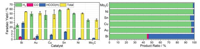
Fig. 3 Left: Column chart indicating the average faradaic yields of  $H_2$  (green), CO (pink), HCOO(H) (blue), and in total (yellow) measured when 20 mL aliquots of 10 mM Cr PDTA were discharged over the heterogenous catalysts Bi, Au, Cu, Sn, Ni, and  $Mo_2C$  inside a sealed  $CO_2$  atmosphere, with error bars indicating the standard deviation within each triplicate set. Right: Row chart indicating relative product ratios for Cr PDTA mediated CO2 reduction over simple heterogeneous catalysts.
