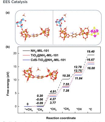
Fig. 11 Energy barrier change diagram for the photocatalytic dehydrogenation of  ${\rm CH_4}$  reforming with the MOF-based composite catalysts.
