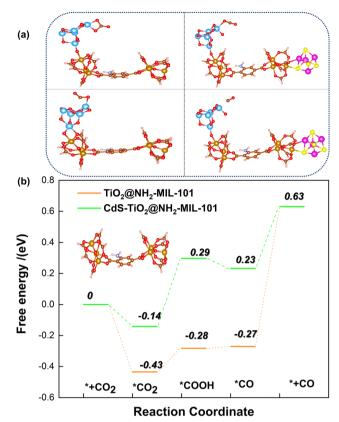
Fig. 10 Energy barrier change diagram of CO<sub>2</sub> to CO photocatalyzed by the MOF-based composite catalysts.
