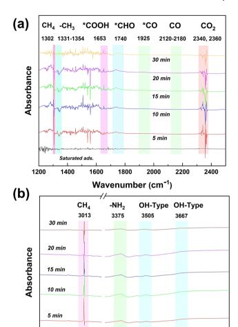
Fig. 12 In situ DRIFTS spectra of chemical substances and intermediates in the photocatalytic  $CH_4$  reforming process by  $CdS/TiO_2@NH_2-MIL-101$  catalysts.
