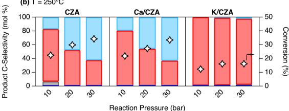
Fig. 4  $CO_2$  conversion (markers) and product selectivity (bars) of CZA, Ca/CZA, and K/CZA in the co-fed  $CO_2$  hydrogenation reaction at (a) T=150-250 °C at 30 bar and (b) P=10-30 bar at 250 °C. Reaction conditions: WHSV of 0.5  $g_{CO_2}$   $g_{cat}^{-1}$  h<sup>-1</sup> and  $H_2$ :  $CO_2$  molar ratio of 3:1. Materials were pre-reduced in 95%  $H_2$ /Ar for 16 h at 250 °C.
