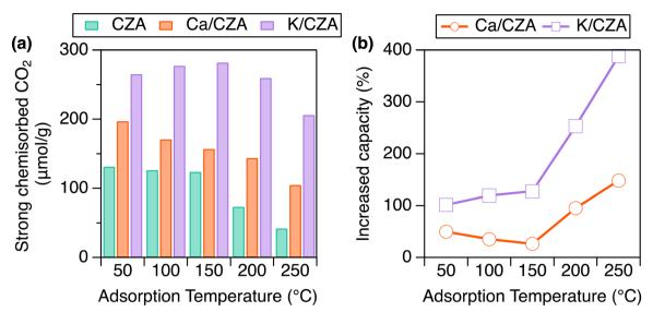
Fig. 2 (a) Strong CO<sub>2</sub> chemisorption values for CZA (teal), Ca/CZA (orange), and K/CZA (purple) at specified temperatures. (b) Increase in strong CO<sub>2</sub> adsorption capacity of the DFMs as compared to parent CZA. Samples were reduced in H2 at 250 °C for 8 h, followed by an 8 h evacuation before analysis.
