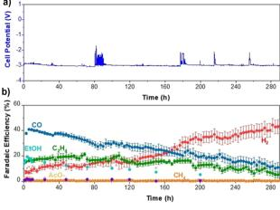
Fig. 10 290 hour  $CO_2$  electrolysis stability test at 60 °C and 200 mA cm<sup>-2</sup>. (a) Potential profile. (b) Faradaic efficiency. Operating parameters were sputtered Cu cathode with 10% be weight MPIP ionomer, MPIP membrane,  $IrO_2$  on carbon anode and 0.1 M CsHCO<sub>3</sub> as an electrolyte. 100 mbar back pressure on the cathode was used as well. Error bars represent the standard error of different injections and measured samples.
