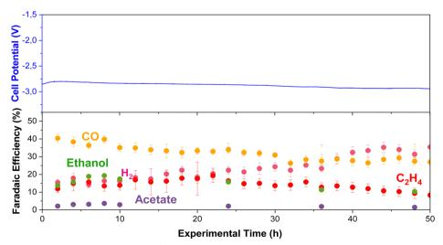
Fig. 9 Long-term stability test at 60 °C and 150 mA cm<sup>-2</sup> using Cu-electrocatalyst. Experimental conditions: Cu-GDE (Cathode), MPIP-AEM, IrO<sub>2</sub> (Anode), CO<sub>2</sub> feeding rate 20 sccm, 0.1 M KHCO<sub>3</sub> as anolyte. Error bars represent the standard error of different injections and measured samples.
