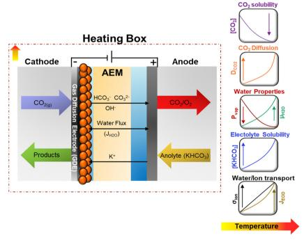
Fig. 1 Schematic representation of temperature dependency on transport and kinetics properties on CO<sub>2</sub>E in zero-gap configuration. Equations for the presented trends for the different properties can be found in the ESI.†
