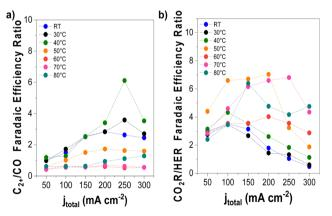
Fig. 4 Selectivity trends as a function of operating temperature and applied current density. (a)  $C_{2+}/CO$  and (b)  $CO_{2-}$ derived products/ $H_2$  FE ratio. Experimental conditions: Cu-GDE (cathode), MPIP-AEM, IrO2 (anode), CO<sub>2</sub> feeding rate 20 sccm, 0.1 M KHCO<sub>3</sub> as anolyte. Results are paired with those presented in Fig. 5.
