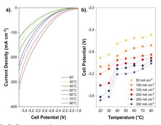
Fig. 3 Temperature effects on the cathode activity through changes in total current density and cell potential at different temperatures: (a) LSV measurements at different cell potentials and (b). Cell potential values as a function of total current density. Experimental conditions: Cu-GDE (cathode), MPIP-AEM, IrO<sub>2</sub> (anode), CO<sub>2</sub> feeding rate: 20 sccm, 0.1 M KHCO<sub>3</sub> as anolyte
