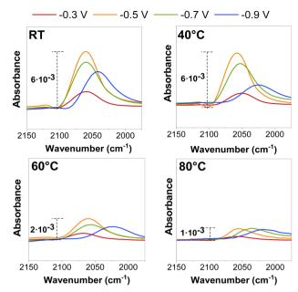
Fig. 2 ATR-SEIRAS CO adsorption peak for electrochemical CO reduction at different potentials (vs. RHE) and operating temperatures. The CO partial pressure for each operating temperature is detailed in Fig. S5 and S6 and estimated with eqn (S12) (ESI†).
