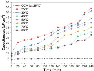
Fig. 7 Tracking the electrode flooding by DLC measurements as a function of the operating temperature at 200 mA cm<sup>-2</sup>. OCV was conducted at room temperature. Experimental conditions: Cu-GDE (Cathode), MPIP-AEM, IrO<sub>2</sub> (Anode), CO<sub>2</sub> flow rate: 20 sccm, 0.1 M KHCO<sub>3</sub> as anolyte.
