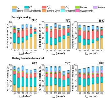
Fig. 8 Effect of the cell heating in the product distribution using two different methods at different operating temperatures experimental conditions: Cu-GDE (Cathode), MPIP-AEM, IrO2 (Anode), CO2 flow rate: 20 sccm, 0.1 M KHCO<sub>3</sub> as anolyte. Error bars represent the standard error of the independent measurements at each different condition.
