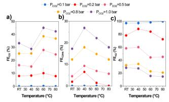
**Fig. 6** Product distribution and faradaic efficiencies of gas products at different operating temperatures and partial pressures of  $CO_2$  (diluted with Ar): (a) CO, (b)  $C_2H_4$ , and (c)  $H_2$ . Experiments were conducted at 200 mA cm<sup>-2</sup>. Error bars represent the standard error of three independent measurements at each different condition.
