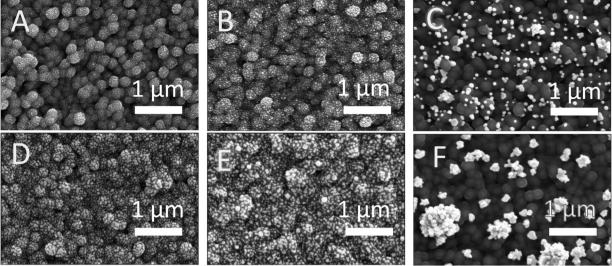
Fig. 5 SEM images of FTO/Au/Sb<sub>2</sub>Se<sub>3</sub>/TiO<sub>2</sub> with Au cocatalyst deposited at different biases -0.4 V (left: A and D), -0.25 V (middle: B and E), and 0.1 V (right: C and F) [referenced vs. Aq/AqCl] and at varying amounts of charge passed in mC cm<sup>-2</sup>: 25 (top: A-C), 75 (bottom: D-F). The scale bar corresponds to 1 µm.
