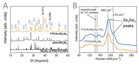
(A) XRD patterns of Sb<sub>2</sub>Se<sub>3</sub> thin films prepared on glass and FTO/Au. (B) Raman spectra of FTO/Au/Sb<sub>2</sub>Se<sub>3</sub> films before and after TiO<sub>2</sub> deposition.
