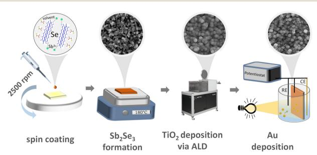
Fig. 1 Schematic representation of the photoelectrode preparation from the Sb<sub>2</sub>Se<sub>3</sub> layer synthesis via spin coating, up to the Au catalyst grafting using photo-electrodeposition, with the corresponding SEM images of the thin films. The illustration for the ink was adopted from ref. 25.
