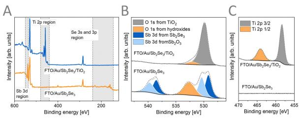
Fig. 3 (A) XPS survey spectra, (B) Sb 3d with O 1s, and (C) Ti 2p high resolution core-level XPS spectra of FTO/Au/Sb<sub>2</sub>Se<sub>3</sub> films before and after TiO<sub>2</sub> deposition.
