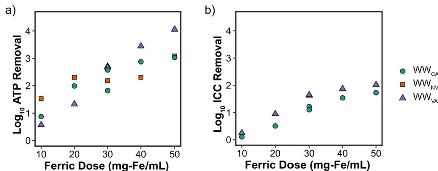
Fig. 3 log<sub>10</sub> removals of (a) total ATP (tATP) and (b) intact cell count (ICC) as determined by flow cytometry, during enhanced coagulation of different secondary effluents. Note: ICC was not measured in Nevada effluent.
