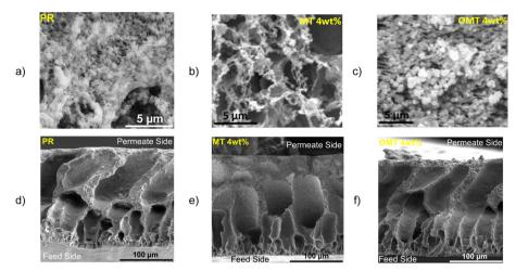
Fig. 2 Surface SEM images (magnification ×8500) of a) pristine PVDF, and MMMs having b) 4 wt% of MT, and c) 4 wt% of OMT; and membrane cross-sections (magnification ×600) of d) pristine PVDF, and MMMs of e) MT and f) OMT at 4 wt% both of each.
