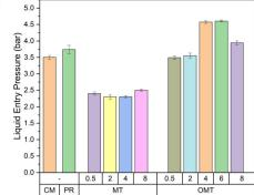
Fig. 5 a) Water CA and b) LEP of fabricated PVDF-clay membranes. Error bars represent standard deviations from three samples.
