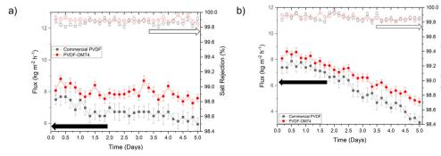
Fig. 7 Long-term stability test of commercial PVDF (black lines) and PVDF-OMT4 wt% (red lines) membranes for permeate flux and salt rejection in presence of only a) NaCl and b) NaCl with HA to promote scaling phenomena. Full and empty symbols represent the membrane flux (kg m<sup>-2</sup> h<sup>-1</sup>) and salt rejection (%), respectively. Error bars represent standard deviations from three samples (or five in the case of the porosity).
