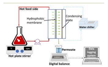
Fig. 1 Schematic diagram of the experimental rig of the AGMD process.
