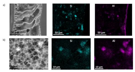
Fig. 3 EDX mapping of Si (center side) and Al (right side) elements for the a) cross-section and b) surface micrographs of PVDF-OMT 4 wt% membrane.
