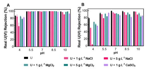
Fig. 3 Comparative uranium rejection by A) NF90 and B) NF270 membranes at different pH levels and ionic conditions. All solutions in these tests contained 150 µg L<sup>-1</sup> of uranium (added as UO<sub>2</sub>(NO<sub>3</sub>)<sub>2</sub>·6H<sub>2</sub>O) and operated at 22 °C and 75 psi. Error bars are included to describe the standard error of the mean.
