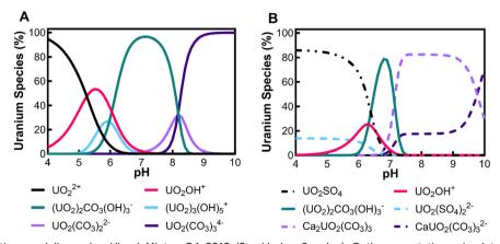
Fig. 2 Uranium speciation modeling using Visual Minteq 3.1 2019 (Stockholm, Sweden). Both computations simulated an open system with carbonate at atmospheric concentrations ( $0.38 \times 10^{-3}$  atm CO<sub>2</sub>). A) Open system uranyl speciation with uranium concentration of 150  $\mu$ g L<sup>-1</sup>, B) open system uranyl speciation with uranium concentration of 150  $\mu$ g L<sup>-1</sup> and CaSO<sub>4</sub> 1 g L<sup>-1</sup>.
