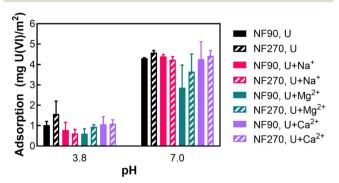
Fig. 4 Comparison of uranium(vi) adsorption by NF90 and NF270 at membrane iso-electric point ( $\sim\!3.8$ ) versus neutral pH ( $\sim\!7.0$ ). All solutions in these tests contained 150  $\mu g~L^{-1}$  of uranium (added as UO<sub>2</sub>(NO<sub>3</sub>)<sub>2</sub>·6H<sub>2</sub>O) and were conducted at 22 °C. pH adjustments were made using 2% HNO<sub>3</sub> and 1 mM NaOH. Error bars are included to describe the standard error of the mean.
