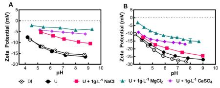
Fig. 1 Streaming zeta potential (mV) scans over pH ranges for A) NF90 and B) NF270 membranes. Additional tests included the addition of ions: UO<sub>2</sub>(NO<sub>3</sub>)<sub>2</sub>·6H<sub>2</sub>O<sub>3</sub>, NaCl, MgCl<sub>2</sub>, and CaSO<sub>4</sub>.
