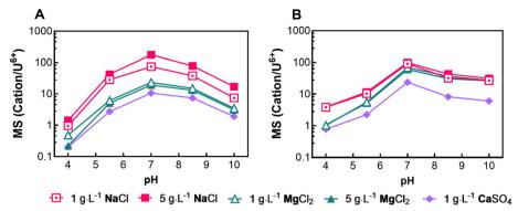
Fig. 5 Membrane selectivity for A) NF90 and B) NF270 based on the transmission ratio of cations to uranium. All solutions in these tests contained 150 μg L<sup>-1</sup> of uranium (added as UO<sub>2</sub>(NO<sub>3</sub>)<sub>2</sub>·6H<sub>2</sub>O) and were conducted at 22 °C. pH adjustments were made using 2% HNO<sub>3</sub> and 1 mM NaOH.
