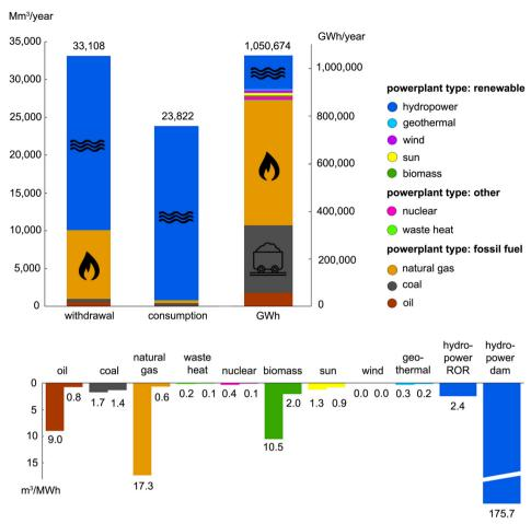
Fig. 1 (Top) Water withdrawal (WW) and consumption (WC) per powerplant fuel for the whole of Africa (in million m<sup>3</sup> per year or Mm<sup>3</sup> per year) as well as the related electricity produced in GWh. (Bottom) Average water intensity (WW and WC) per powerplant fuel for Africa (in m3 MWh-1). Note that these are average values for all 2534 power plants, whereas individual plants show a wide range (range of values shown in Table 3).
