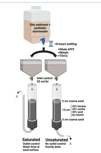
Fig. 1 Diagram of experimental setup showing synthetic stormwater generation, inflow, engineered media description, and saturated and unsaturated conditions
