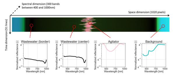
Fig. 1 Top: typical data-cubes (normalized) with pseudo-RGB colouring corresponding to 380 nm, 500 nm, and 900 nm. One line consists of 1020 pixels, which have a spatial resolution of about 0.1 mm. The image consists of 51 lines collected in 10 seconds. Each image's pixel contains a spectrum ranging from 400 to 1000 nm. Bottom: the spectral dimension is visualized to show the differences between various image areas.
