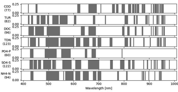
Fig. 6 Number of selected wavelengths (left, in brackets), PLS weights (dots), and selected wavelengths (grey vertical lines) for each pollution variable. Some patterns are recognizable, but their interpretability is limited (see 3.6).
