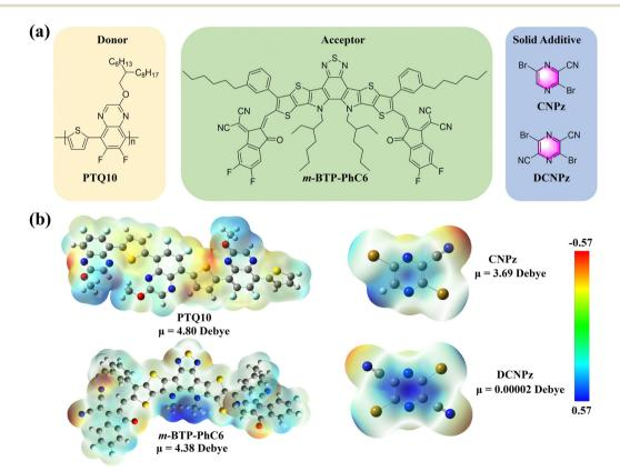
Fig. 2 (a) Chemical structures of polymer donor PTQ10, acceptor m-BTP-PhC6, and solid additives CNPz and DCNPz. (b) ESP distributions and dipole moments for PTQ10, m-BTP-PhC6, and the two solid additives.
