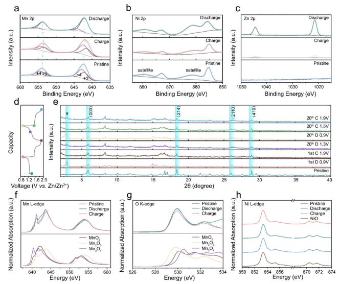
Fig. 7 The charge storage mechanism of  $V_m$ -NMO batteries. Ex situ XPS profiles of  $V_m$ -NMO at different states: (a) Mn 2p. (b) Ni 2p. (c) Zn 2p. (d) and (e) Ex situ XRD profiles of V<sub>m</sub>-NMO at different states. (f) Mn L<sub>3,2</sub>-edge NEXAFS profiles at different states. (g) O K-edge NEXAFS profiles of cathode materials in different states. (h) NEXAFS profiles of Ni L-edge of cathode materials in different states.
