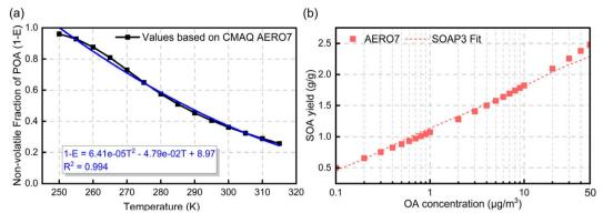
Fig. 2 (a) Polynomial fitting between particle fraction of POA (1 – E) and temperature with  $C_{OA} = 50 \mu g m^{-3}$ ; (b) fitting of SOAP3 SOA formation from SVOCs to AERO7 over a range of total OA concentration from 0.1 µg m<sup>-3</sup> to 50 µg m<sup>-1</sup>
