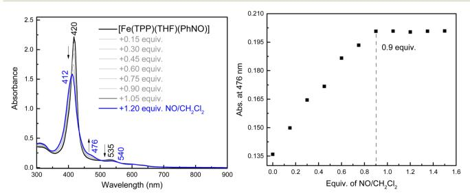
Fig. 8 UV-Vis spectra of the titration of ~14 μM [Fe(TPP)(THF)(PhNO)] (black) in THF with a NO-saturated solution of dichloromethane, forming the ferrous NO complex [Fe(TPP)(NO)] (blue). Right: Changes in absorbance at 476 nm upon addition of the NO solution, showing that the reaction is complete after the addition of ~1 equivalent of the NO-saturated dichloromethane solution.
