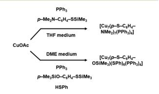
Fig. 3 Process to synthesize similar Cu atom containing two different thiolates protecting NCs.
